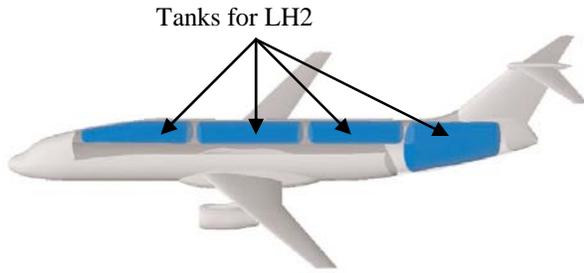
**Fig.5. LH<sub>2</sub> tanks storage scheme of "Cryoplane" project [10]**
