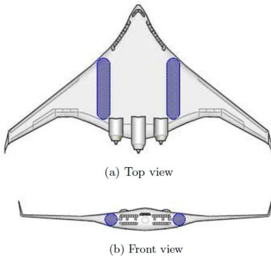
**Fig. 6. A possible BWB layout with LH<sub>2</sub> tanks.**
