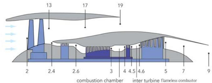
**Fig. 9. Engine Layout and Numbering [22]**
