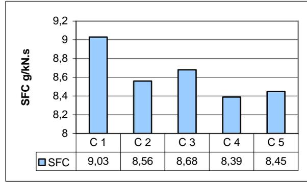
Fig. 13. SFC comparison for various engine configurations at take-off
