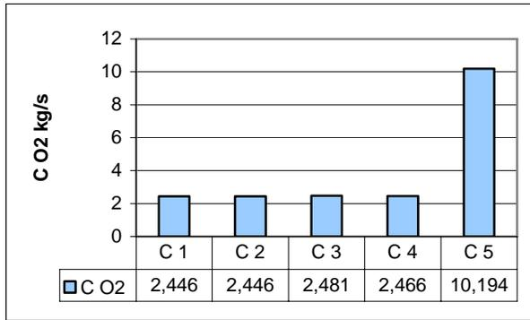
**Fig. 15. Reduction in CO2 emission for various engine configurations at take-off**
