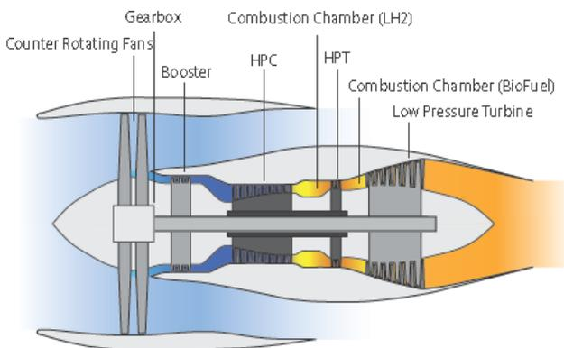
**Fig. 7. Proposed Engine Layout**
