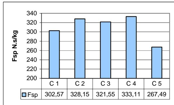
Fig. 14. Specific thrust comparison for various engine configurations at take-off
