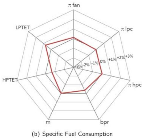
**Fig. 10. Sensitivity analysis of various design parameters on hybrid engine (a) Specific thrust (b) SFC**
