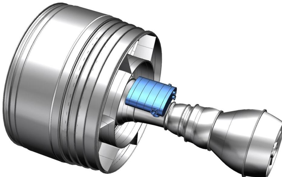
**Figure 7** Hybrid engine 3D mock-up with basic model of the heat exchanger (Source WSK PZL Rzeszow).
