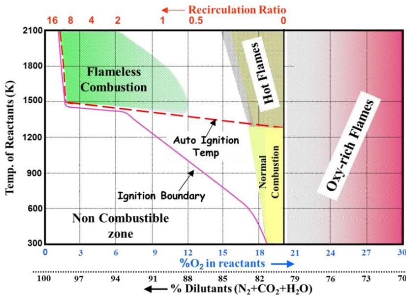
**Figure 10** The principle of flameless combustion (Source Technion)
