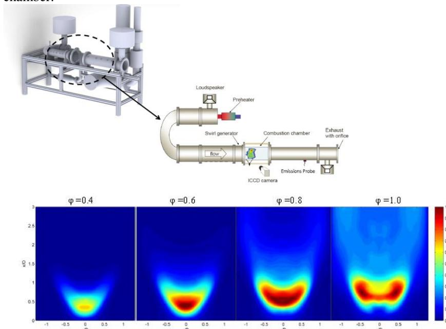
**Figure 9:** Abel-deconvoluted time-averaged OH\* images normalized by maximum intensity of  $\phi=1$ , indicating location of heat release. Images recorded at a mass flow of 180 kg/h and an inlet temperature of 620 K for configuration with long mixing tube and high swirl. (Source TU Berlin)
