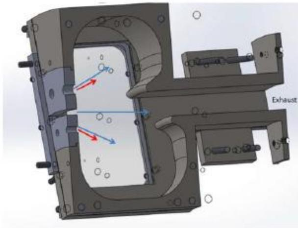
**Figure 11:** Side view of test article showing air (blue) and fuel(red) inlets, upper and lower cavities and the exhaust.
