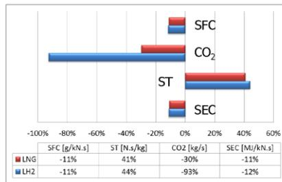
Comparison of hybrid engine with PW4056
