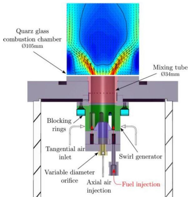
Applying aerodynamic, swirl-induced, vortex breakdown flame stabilization takes away the necessity of a bluff body or centre body which would potentially suffer from material degradation due to the high flame temperatures of hydrogen flames. Accordingly, in the current study, a cylindrical mixing tube without centre body is used in order to further enhance mixing. The swirling flow downstream of a mixing tube or
