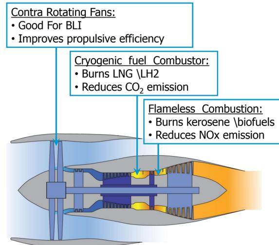
Figure 6: Schematic of the multi-fuel hybrid engine.
