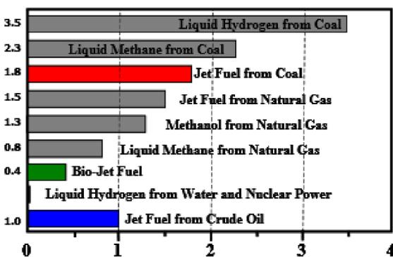
Figure 3: Relative life cycle CO<sub>2</sub> emission for various fuels compared to jet fuel [2].
