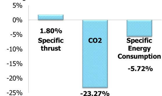
Figure 7: Comparison of the AHEAD hybrid engine to GE90-94B.
