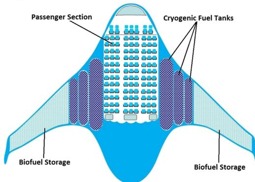
Figure 5: Schematic of the multi-fuel BWB concept
