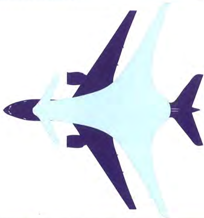
Figure 6. Comparison of the BWB with a Boeing 777-200ER
